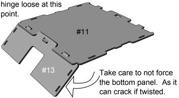
Step 12: Insert the right side panel (#15) by first engaging the hook tabs into the botttom panel (#13) working your way around the
