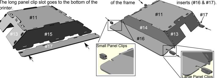
Step 16: Install the assembled front and back bays onto your printer using the panel clips to engage the printer frame and secure the front and back bays in place.
