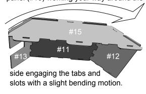
**Step 14:** Attach the left side frame insert (#17) The long panel clip slot goes to the bottom of the
