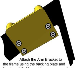
the frame using the backing plate and four long M3x20 machine screws supplied.
