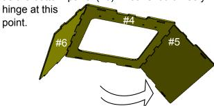
**Step 13:** Repeat with the left side panel (#7). Be sure to engage the hooks in the bottom panel (#6) first.
