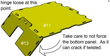
Step 18: Insert the right side panel (#15) by first engaging the hook tabs into the botttom panel (#13) working your way around the
