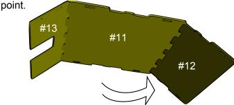
Step 19: Repeat with the left side panel (#14). Be sure to engage the hooks in the bottom panel (#13) first.
