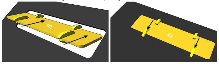
**Step 9:** Install the Right Side Panel (#3) into the opening on the right side of the printer's frame, just as you did for the Left Side Panel (#2). Removing the panels is simply the reverse of installation.
