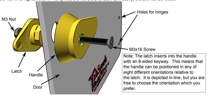
**OPTIONAL:** You may choose to reverse the door, and have the hinges on the left, if you wish. To do so, just flip the door when installing the handle, latch and hinges. You must also flip the Front Face Plate (#4), so that the hinge holes are on the left when assembling the front panels.
