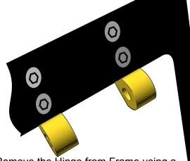
Remove the Hinge from Frame using a 2mm hex wrench to remove the four flat head M3 machine screws.
