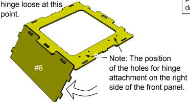
**Step 12:** Insert the right side panel (#8) by first engaging the hook tabs on the botttom panel (#6) into the slots on the side panel (#8)
