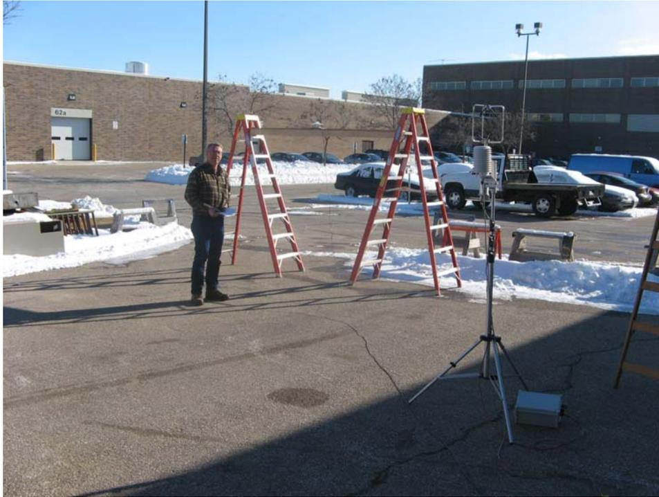
**Figure 25** Total radiation on horizontal measurements, picture in direction south-east, ground partly snow covered, © Thomas Kaminski
