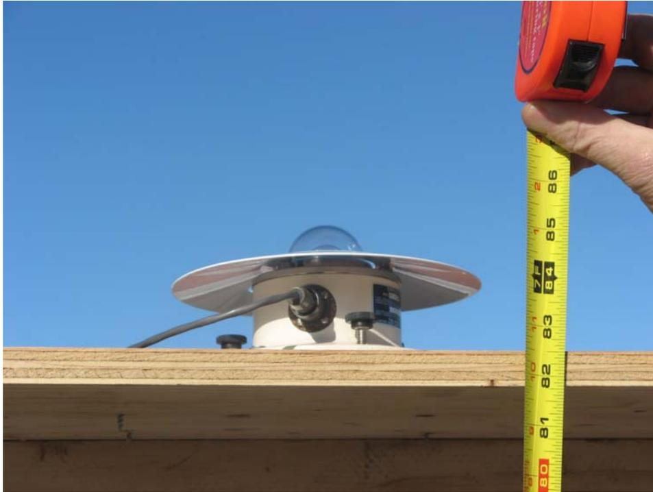
**Figure 27** Total radiation on horizontal measurements, picture of pyranometer and measure showing height above ground, © Thomas Kaminski
